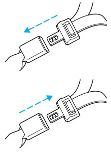
2. To unfasten, push the release button and remove the tongue from the buckle. The front and rear outboard safety restraints in the vehicle are combination lap and shoulder belts. The front and rear seat passenger outboard safety belts have two types of locking modes described below:
